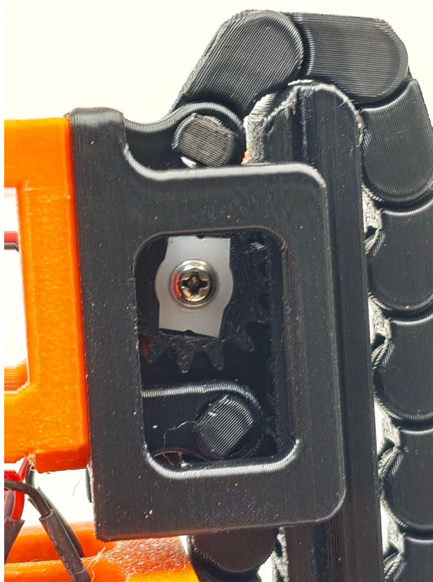
Tighten screw(Shorter one from the servo kit).
