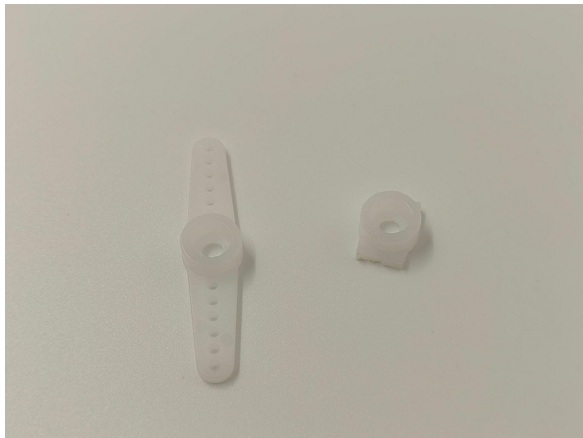
Cut the first hole of the servo's attachment part, insert into gear hole
