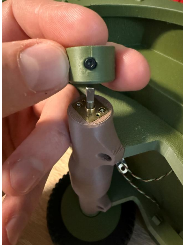
Screw the rear wheel adapter to the motor BT2x6 (2x) Make sure that the screw is screwed onto the flat side of the motor shaft. Only tighten lightly!!!
