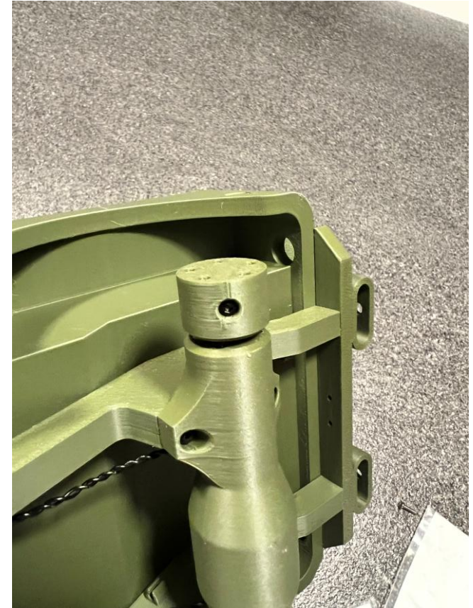
Screw the rear wheel adapter to the motor BT2x6 (2x) Make sure that the screw is screwed onto the flat side of the motor shaft. Only tighten lightly!!!
