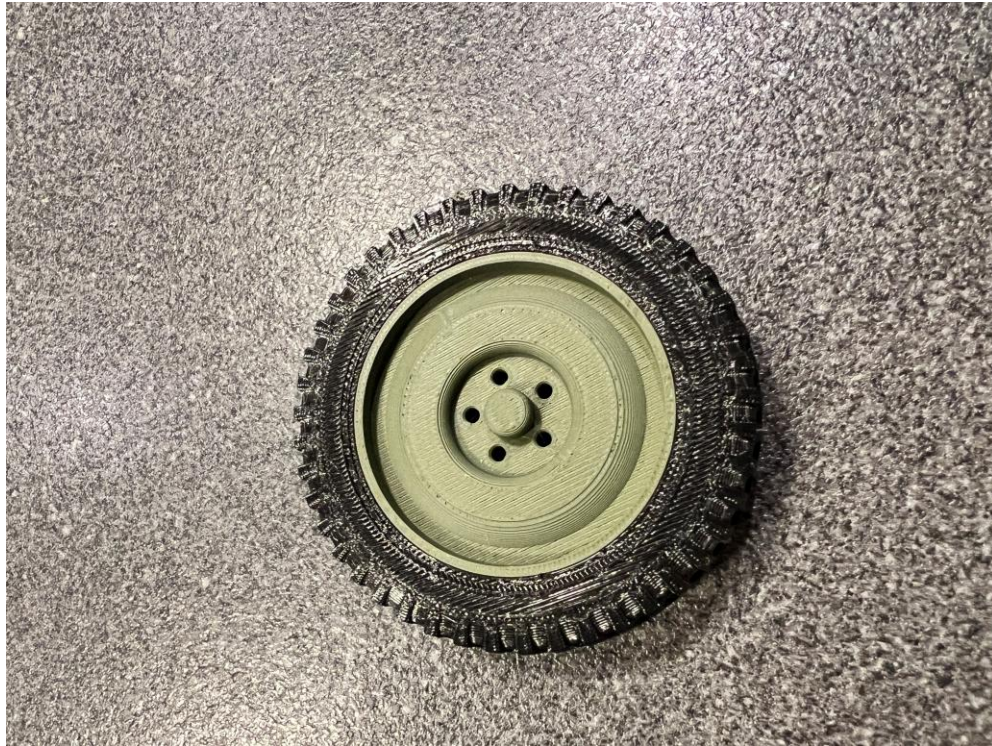
Tire TPU version press on rim. For PLA version gluing
