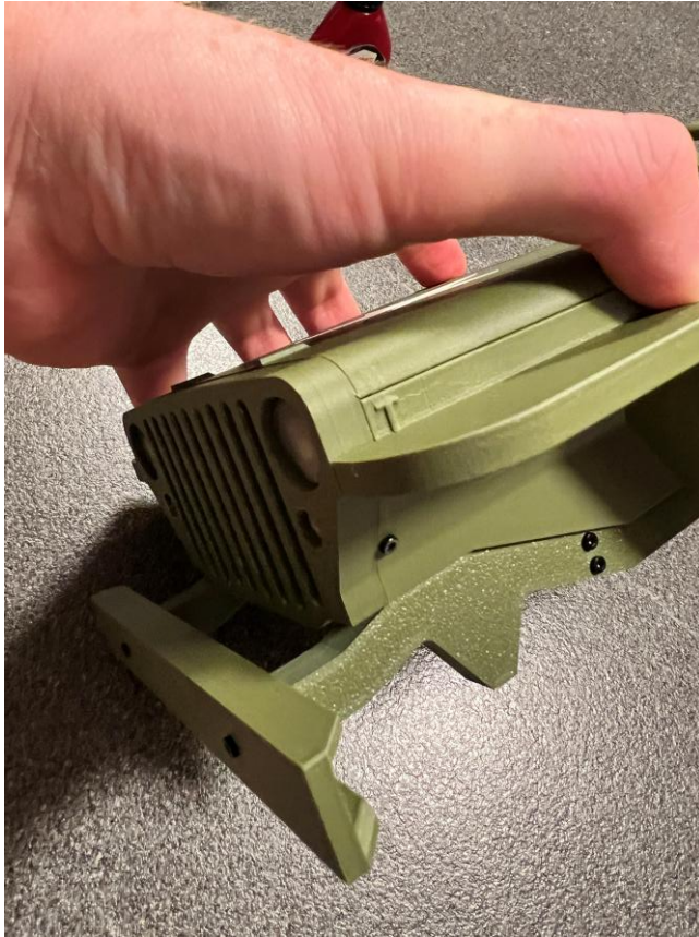
Screw the radiator grille to the front body BT2x6 (2x)
