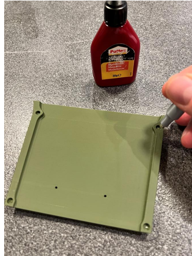
Glue 4x magnets (4x2mm) into the hood)
